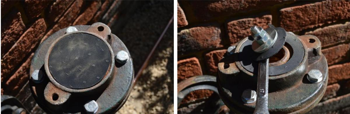
Having ordered a new bucket/valve from Robinson & Sons, it was obvious that the operating rod (also threaded to M10 x 1.5) was too long for the barrel, and we would have to fabricate a new linkage in any event. A yoke was made up from flat steel strip with a hole at the top for the operating
